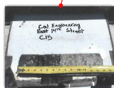
EAST 14TH STREET - CORE #15 HMA Layer 7" AB Layer 3.5" PCC Layer 7"
