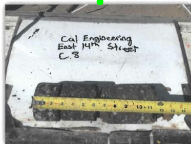
EAST 14TH STREET - CORE #8 HMA Layer 11.5" AB Layer 7" PCC Layer 0"
