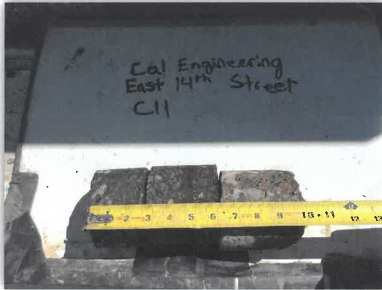
EAST 14TH STREET - CORE #11 HMA Layer 6" AB Layer 5" PCC Layer 4"
