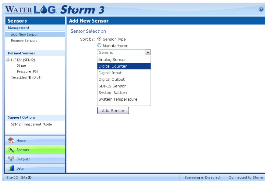
Figure 7) Adding a digital counter for a tipping bucket rain gauge
