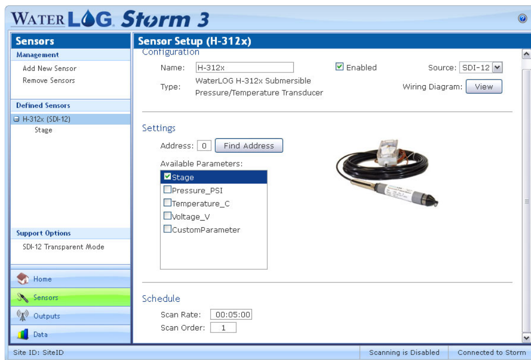
Figure 5) SDI-12 pressure transducer setup
