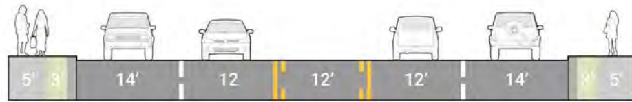
Roadway Before Narrowing
