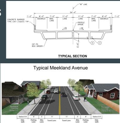
Sidewalk and permeable concrete widths vary based on available Right-of-Way
