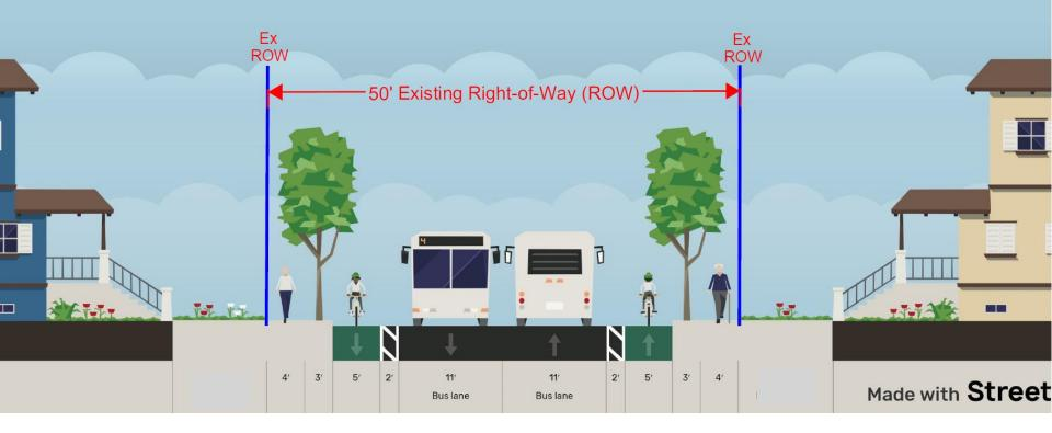
This typical section shows the project features for Alternative #3. The dimensions shown are preliminary and may change to accommodate local site conditions.
