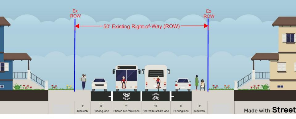
This typical section shows the project features for Alternative #1. The dimensions shown are preliminary and may change to accommodate local site conditions.
