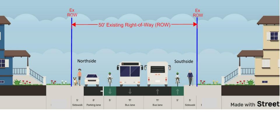
This typical section shows the project features for Alternative #2B. The dimensions shown are preliminary and may change to accommodate local site conditions.
