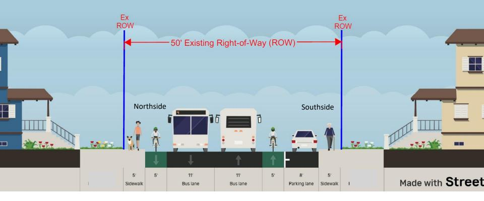
This typical section shows the project features for Alternative #2A. The dimensions shown are preliminary and may change to accommodate local site conditions.
