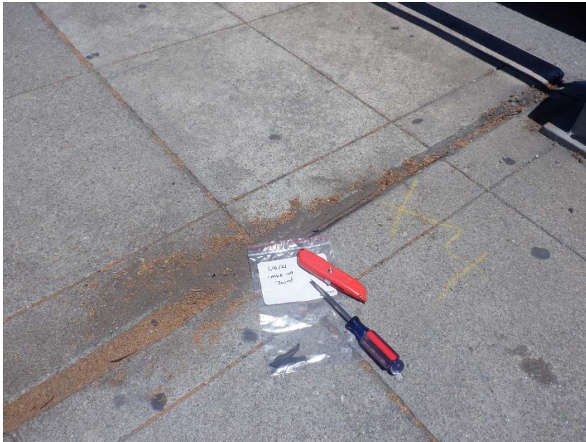
Photo 8. ACM sample MKA-09 from the joint material in the expansion joint along the sidewalk on the west side of the bridge.
