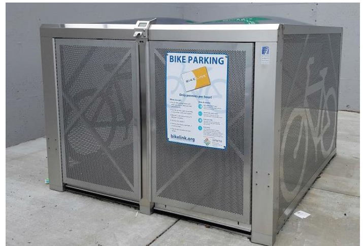
Figure 4.11. Bike lockers are an example of long-term, secure bicycle storage.
