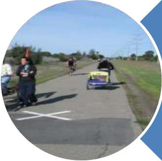
**Shared Use Paths (Class I)** are two-way paved facilities, physically separated from motor vehicle traffic and used by bicyclists, pedestrians, and other non-motorized users. Shared use paths are often located in an independent alignment, such as a greenbelt, flood control channel park, or abandoned railroad.
