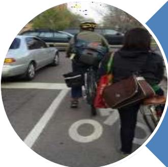
**Bike Lanes (Class II)** provide an exclusive space for bicyclists in the roadway. Bicycle lanes have established painted lines and symbols on the roadway surface. Bicycle lanes are for one-way travel and are typically provided in both directions on two-way streets and/or on one side of a one-way street.
