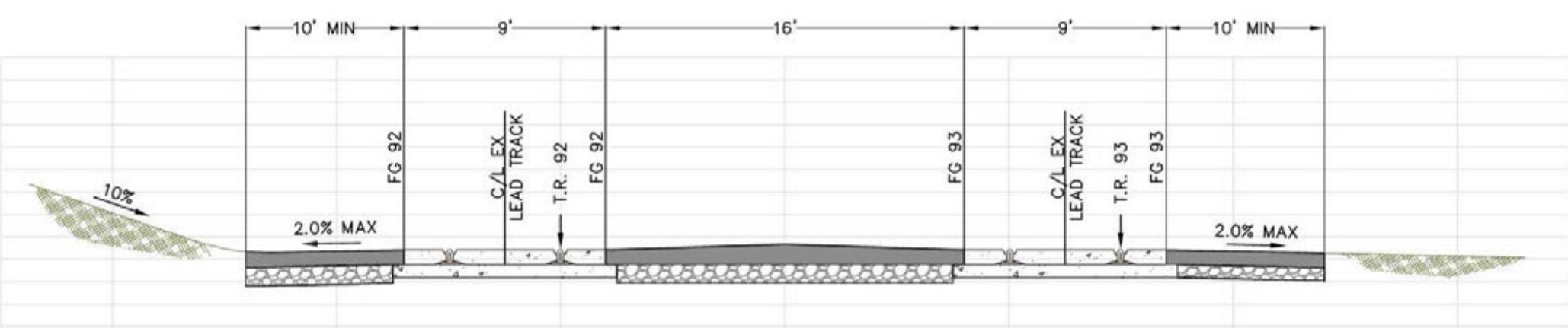
Figure 2-2 – At-Grade Crossing Cross Section
