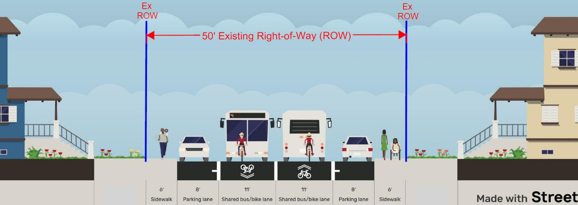
*This typical section shows the project features for Alternative #1. The dimensions shown are preliminary and may change to accommodate local site conditions.*
